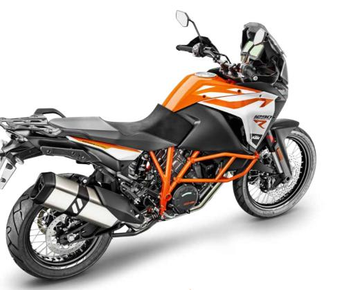
ENGINE 2-CYLINDER, 4-STROKE, V 75° DISPLACEMENT 1.301 CC 118 KW (160 HP) @ 8.750 U/MIN TRANSMISSION 6 GEARS FUEL CAPACITY APPROX. 23 L DRY WEIGHT APPROX. 217 KG
